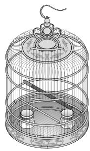
Insert the slotted perch ends into the vertical cage wires. Let the perch rest on the heavy horizontal bar for stability.
