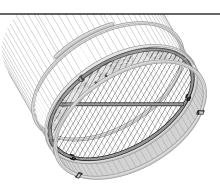
Insert the grille at an angle to bypass the base tray clips along the bottom rim. Push the grille up and into the grille holding clips.
