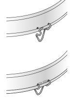
Insert the wire tray clip into the holes along the bottom lip of the cage body.
