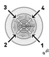
Finial attaches to the roof in four places. Hold the nut in place on the inside and, from the outside, screw in the phillips head screw.
