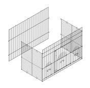
Create the cage body by beginning at the bottom corner and hooking the panels together (arrow #1). Weave the alternating hooks together up the seam by flexing the mesh panels (arrows #2-5).
