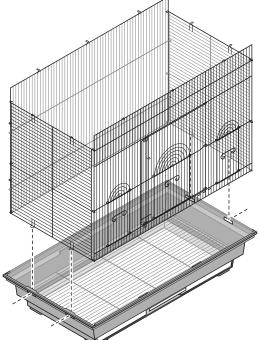
Add the assembled mesh to the base, by inserting the extended loops along the sides into the open slots on the base.
