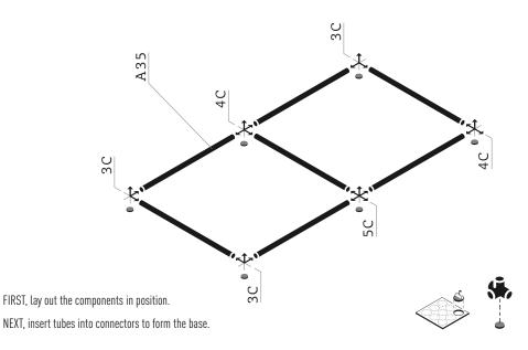
Self-adhesive foam pads (if used) should be placed on the underside of all connectors.
