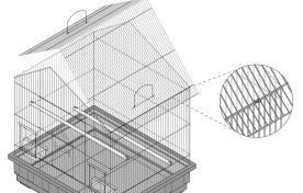
Start at one end. Catch the inset horizontal wire on the roof mesh under the loops on the side panel.
