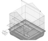
Insert the perches on a vertical wire, resting on a horizontal wire for stability.
