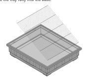
Set the assembled mesh into the base. Guide the loops on the side panels into the holes along the lip of the base.
