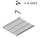
Start at one end. Attach the leg frame rails together
