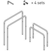
Start with the UPPER holes first. Attach the frame legs together with the washer and bolt on the outside and the <u>nut</u> on the inside.
