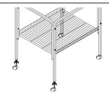
Fully insert the post of the casters into the holes in the base of all four frame legs.
