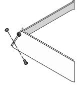
To make assembly easier, flip the FRONT and SIDE guard upside down on the floor as shown.
