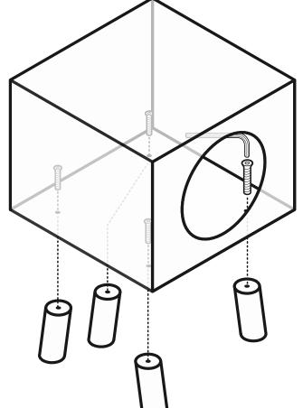
Tighten screws snuggly to create stable connections.
