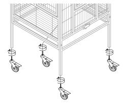
Screw the threaded caster post into the frame leg at each corner. If preferred, tighten each caster with a slim wrench.
