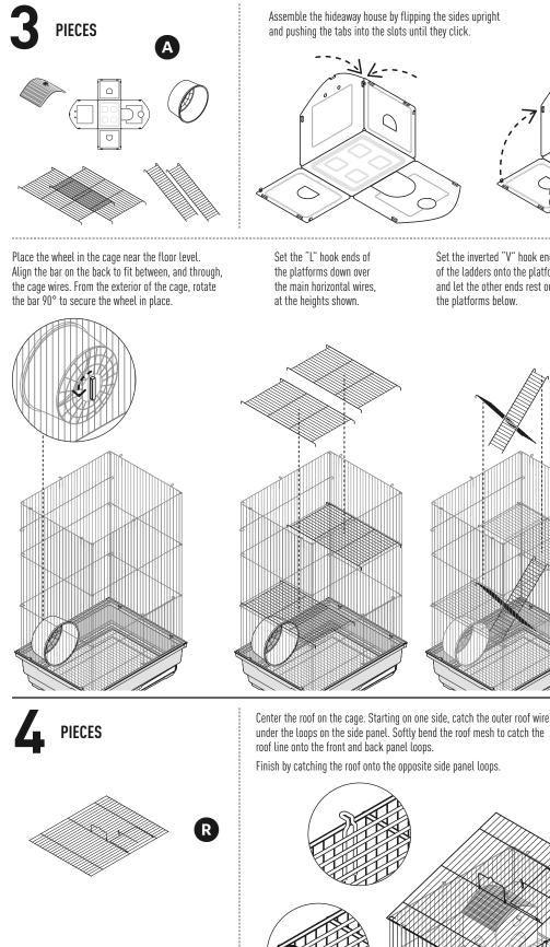
Align the pegs on the underside of the roof into the slots on the side walls until they click in place.
