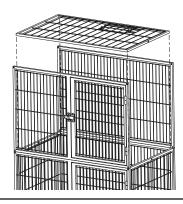
Secure the grille with a short screw on each side.
