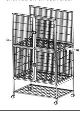
First, slide the upper side panels into place. Next, secure the panel intersections with long screws at all corners.
