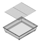
Set the grille into the base. Push the tray into the base.
