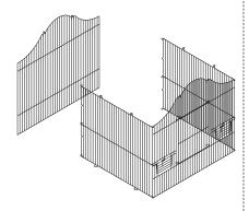
Attach the back panel to the right-side panel: Start in the lower corner. Hook the right-side panel onto the back panel.
