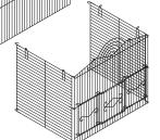
Attach the back panel to the three-panel unit: Start in the lower corner. Hook the right-side panel onto the back panel, then weave the alternating hooked wires of the two panels together, up the seam, to the top.
