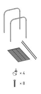
Lay one side frame on its side, attach the storage shelf with a hex screw, then add and attach the opposite side frame.
