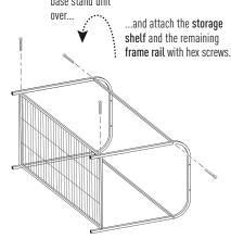
With the cage still on its side, add the **rolling casters** into the frame legs. Set the completed stand unit aside.
