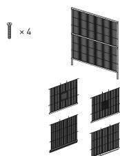
Orient the **lower side panel** with the grille/tray track facing the cage interior and the open end facing the cage front.
