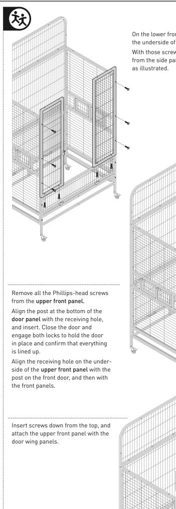
On the lower front panel, remove the screws from the underside of the top frame rail.
