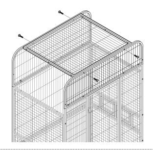
the panels for the remaining screws. Finish attaching the upper side panels with the remaining screws.
