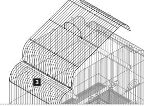
Then catch the roof on the loops along the front and back panels.
