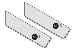
Pre-assemble in pairs (SG1 + SG2) and (SG3 + SG4).
