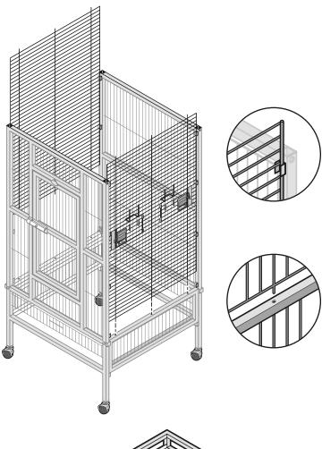
Insert the corner posts at the base of the roof frame into the open corners on the cage frame.
