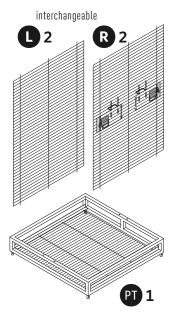
The side panel with cup doors can be inserted on either the left or the right side. Be sure the doors will swing open to the cage exterior.
