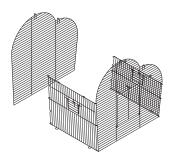
Attach the back panel to the rightside panel:
