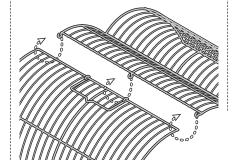
With the roof assembled, catch the bottom horizontal wire of the roof under the loops on the side panel. Softly bend the roof mesh to catch the roof line onto the front and back panel loops. Finish by catching the roof onto the
