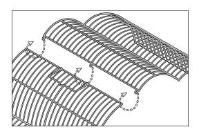
With the roof assembled, catch the bottom horizontal wire of the roof under the loops on the side panel. Softly bend the roof mesh to catch the roof line onto the front and back panel loops. Finish by catching the roof onto the opposite side loops.
