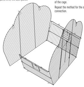
Going up the seam, continue catching the hooks around from the outside while keeping the notched portion of the wire to the interior
