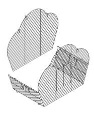
Attach the back panel to the rightside panel: Start in the lower corner. Hook the right-side panel onto the back panel.
