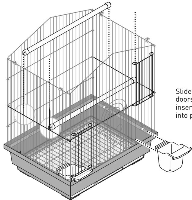
Slide the cup doors up and insert cups into place.
