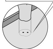
On the underside of the base and of the trunk, you will find handwritten "1" and "2" marks. All of these markings will help you with correct placement of the trunk on the base.
