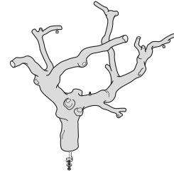
With a crescent wrench or socket wrench with  $\frac{1}{2}$ " (12 mm) socket, completely remove the bolt and washer from the base of the crown.
