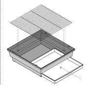
Set the assembled cage body into the base.
