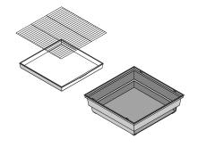
Place the **grille** down into the base and slide the **tray** in from the front.
