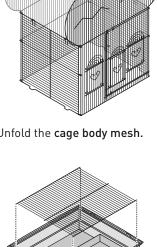
Prepare the **base** by placing the grille down into the base and sliding the **tray** in from the front.
