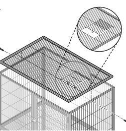
Place the roof (CR - with the non-removable sliding door) in position and attach with a hex screw on each end.
