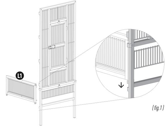
Slide the tabs on the **left side lower (L1)** panel down into the sleeves on the legs of the **front (F)** and **back (B)** panels.
