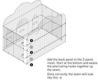
Weave the panels together on the remaining seam by the same method.
