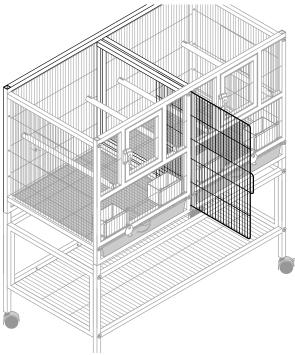
Leave the center **divider grille** out for full-cage use, or slip it in place to divide the cage interior into two separate spaces.
