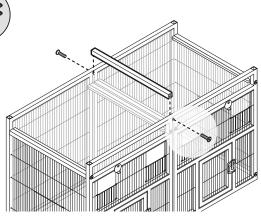
method, securing all panels together with hex screws.
