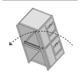
Install the two remaining square rails. Secure the rails with hex screws.
