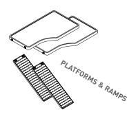
• Hook the ramps onto the underside of the • Insert the **platforms** into the cage (lower platforms first. platform/ramp first). Set the extended tabs over horizontal wires at an equal height along the front and back. Push tabs down onto the wire to lock the  $% \left( 1\right) =\left( 1\right) \left( 1\right$ platforms in place.
