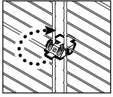
• Flip the connector up and click it onto the vertical wires, above and below the horizontal wire.
