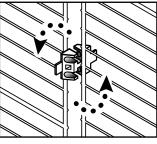
Insert the connector between the panels and twist 90°.
