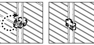
• Connect all panels together with the cage connectors; four along each corner seam. ٠ • Make sure the front panel is assembled so that the Heavy vertical wires door opens out. face cage exterior
