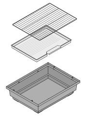
Place the removable grille into the base and slide the pull-out tray into the opening.
