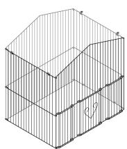
Weave the front panel/left side seam together using the same method to create the cage body.
