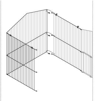
Add the right side panel to the back panel. Start at the bottom and fully pull the "R" hook over the vertical wire. Continue up the seam until all are fully linked.
