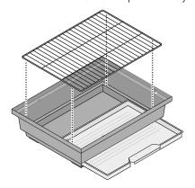
Set the assembled mesh into the base. Hook the side panels up under the extended plastic tabs along the rim of the base.
