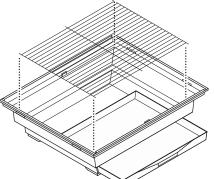
Place the removable grille into the base and slide the removable tray into the opening.
