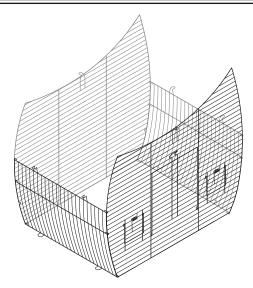
Starting from the bottom, catch the extended hooked wires of the side panel onto the back panel. The notched wire stays on the interior of the cage and acts as a backstop against the pull of the hooked wires.
