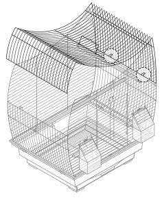
Starting on one end, catch the roof on the looped hooks along the side.
