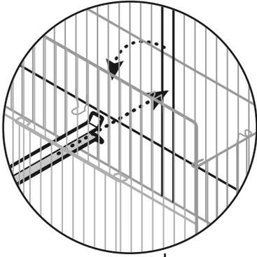
Rest the **divider channel** down onto the horizontal wire in front and back.
