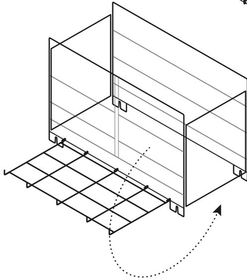
Rotate the base grid around to the cage underside and catch the hooks over the bottom horizontal wire.
