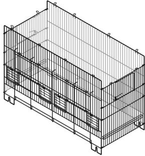
Unfold the cage body to create a box shape.
