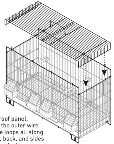
Add the **roof panel**, catching the outer wire under the loops all along the front, back, and sides of the cage body.
