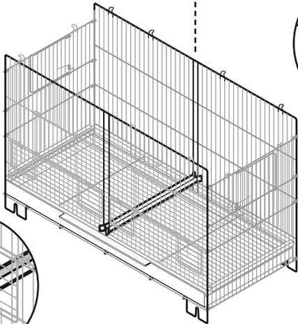
Starting from the cage exterior, insert the **perches** sideways and then rotate 90°, trapping the cage wire between the perch bracket and base.
