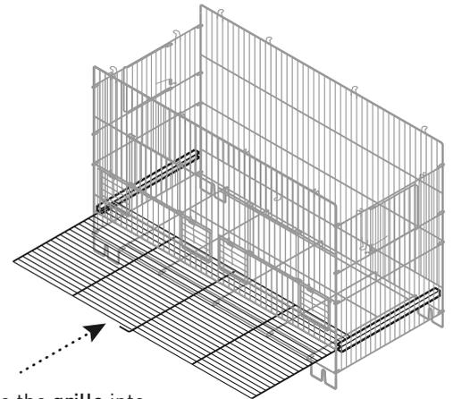
Slide the grille into the tracks, resting on the looped wire at the back.
