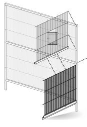
Confirm the <u>cup door</u> on the **upper side panel** opens out.
