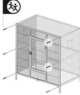
If you have an assistant, have them hold the unit upright. Align all <u>extended wires</u> of the **roof/side** panels with holes on the **front panel** frame.
