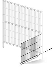
Align the <u>extended wires</u> on the **lower side panel** with the <u>holes</u> on the **back panel** frame.
