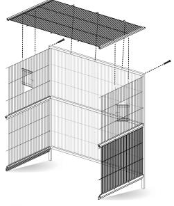
Align extended wires along the <u>back</u> <u>edge</u> of the **roof panel** with holes on the back panel frame. Align extended wires along the <u>side panels</u> with holes on the underside of the roof frame.
