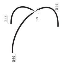
When building the hideaway arch, insert long tubes into the sleeves of the fabric piece first, then add the connectors.
