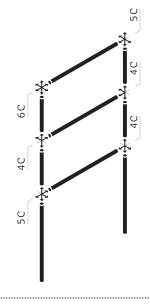
Begin with assembly of the lower portion and build up with each stage.
