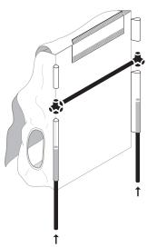
Build and add the components first, then secure the velcro sleeve around the horizontal tube.
