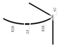
Make two hideaway corners. Both are exactly the same and use duplicate components.
